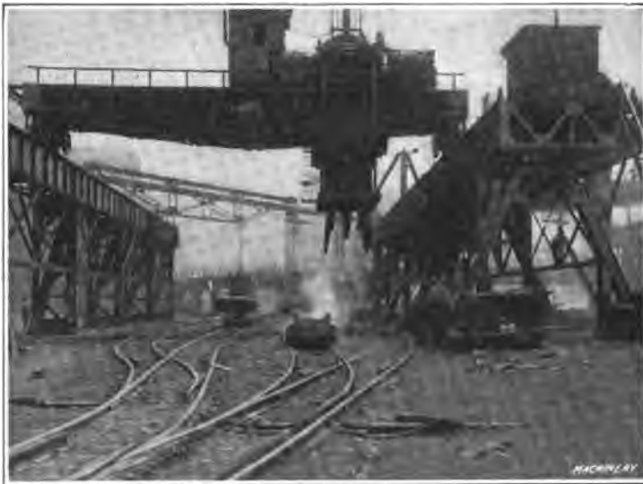
Fig. 3. Electric Stripper for Removing Mold from Ingot
